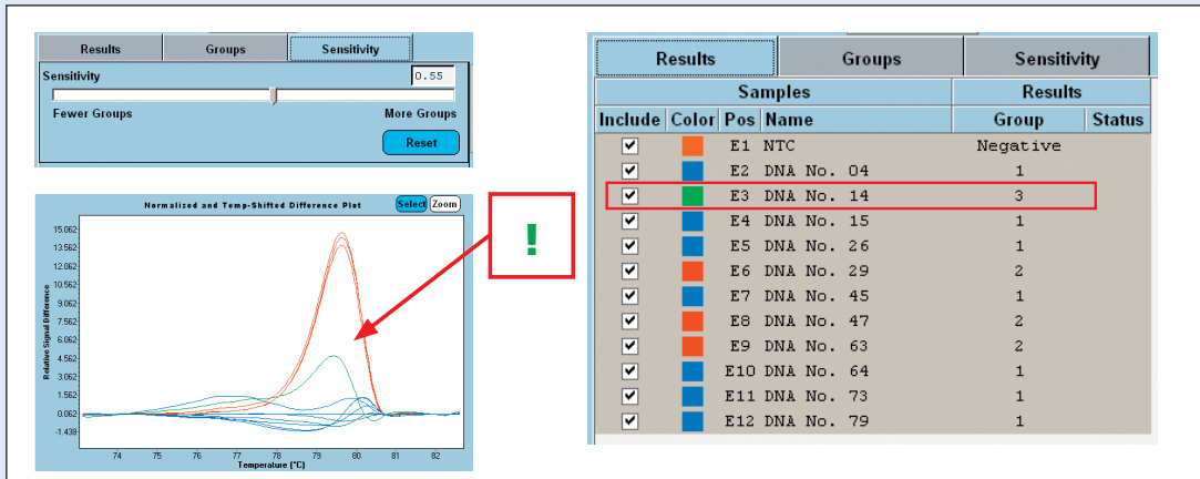
Figure 12b: Changing the sensitivity setting clarifies the situation. The sample of interest is now shown as sequence variant in the result list!
