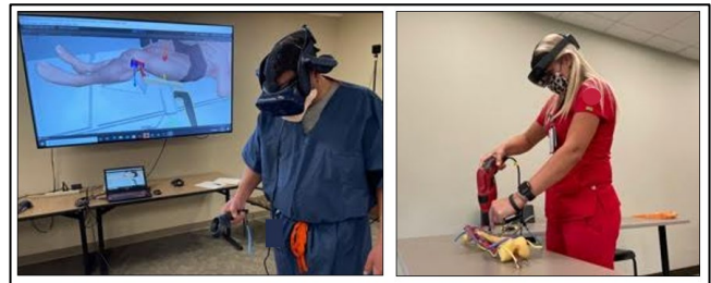
Fig. 4. Users interacting with the VR based environment using Vive Pro headset (left) and MR based environment using HoloLens 2 and physical mockup (right)
